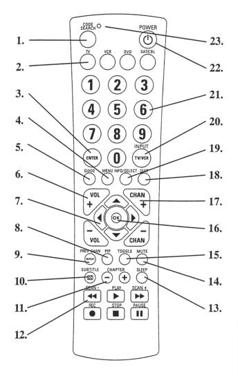
Note: The **REC** button must be pressed TWICE to record from your VCR. For some brands of VCRs, you might need to press the **REC** button once, then press it again for three seconds.
