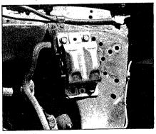
3. The stock small-block V-8 mount positioned in the factory mounting holes prior to slotting of the holes. When the big Rat was lowered into position, it failed to rest fully on the mounts, but rather than waste time looking for different motor mount cups, the holes were slotted to give the additional clearance the big-block needed.
