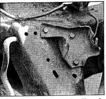
2. Chevy has sufficiently offset the frame mounts for the little V-6 so that the engine has the same relative position in the engine bay as the V-8. This eliminates any transmission/clutch alignment problems. It also makes for universal positioning of the clutch cross-shaft stud on the various blocks.
