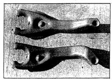
7. Above—clutch arm from older supercars, Part No. 340278. Below—clutch arm from the El Camino, designed for an offset stud and bent to provide more clearance for the adjustment rod.
