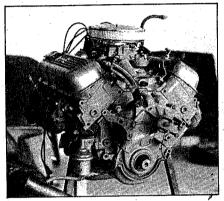
1. A \$100 "smoker" from the salvage yard, that, except for a slightly warmed-up camshaft, is stock down to its low-profile intake and Rochester Q-Jet. But don't let that fool you, because by today's standards, it will still pump out neck-jerking horsepower.
