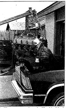
9. The moment of truth. The big Mark IV is lowered into the engine bay of the El Camino for a test fit. The Saginaw three-speed is mounted behind a rebuilt 11-inch factory clutch.
